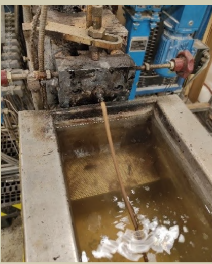
Die output with hop-based composite filament
