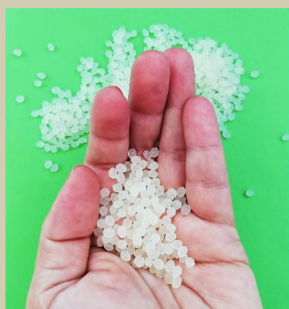
Bio-based polymer to be mixed with the treated hop fibers from ZELFOS
