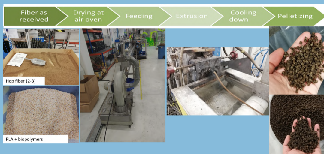
Full extrusion-compounding process followed at TECNOPACKAGING from the reception of the fibre to the production of the hop-based bio-composite.
