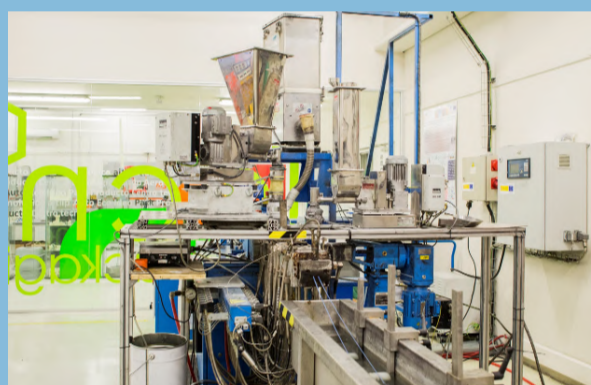
Extrusion compounding Coperion ZSK 26 twin-screw machine used for the production of bio-composites.
