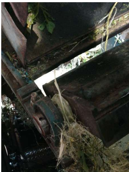
Figure 11: The twine curled around the axle
