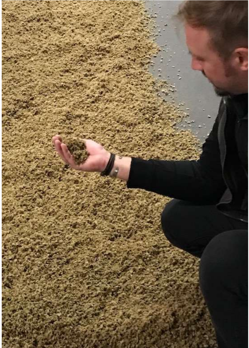
Floor drying of Hops/PLA processed fibres.
