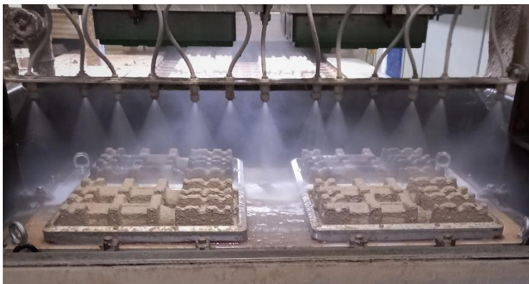
Forming of trays and transferring to the belt
