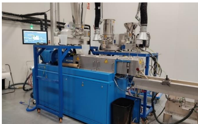
Compound extrusion machine (COPERION)
